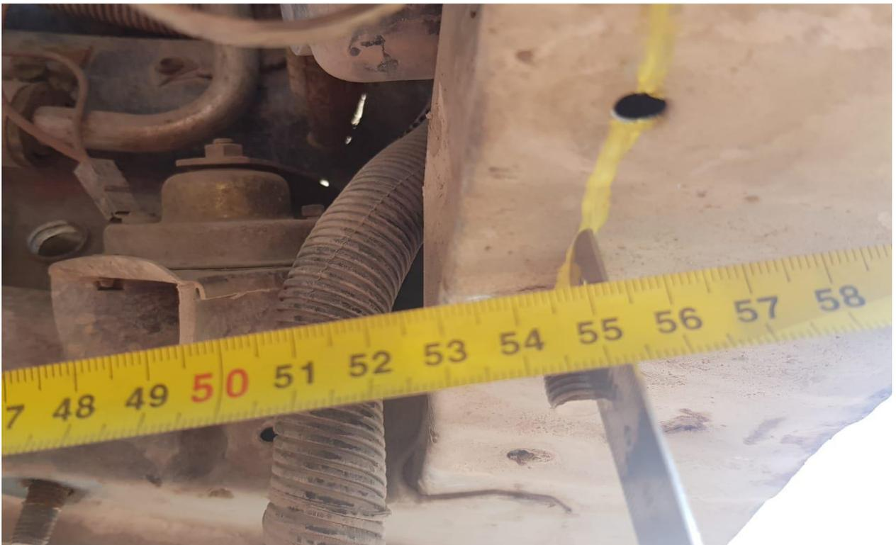
**MEDIDA LARGO DE ANCLAJE DE BRAZO PARRILLA DE SUSPENSION A FRENTE INFERIOR DE CARROCERIA (550 MM).**
